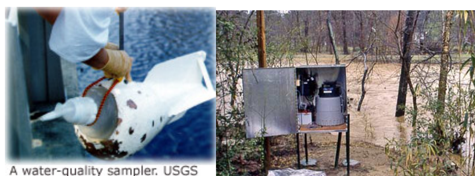
Figure 23- Left: Depth integrating water quality sampler. Right: Autosampler that can be set to sample at fixed time intervals, or flow levels
