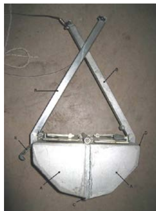
Figure 27 – Grab for sampling invertebrates in deeper-water areas
