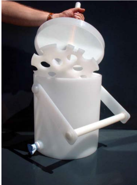
Figure 17 – Suspended sediment and water quality churn splitter used to accurately subsample composited suspended sediment samples
